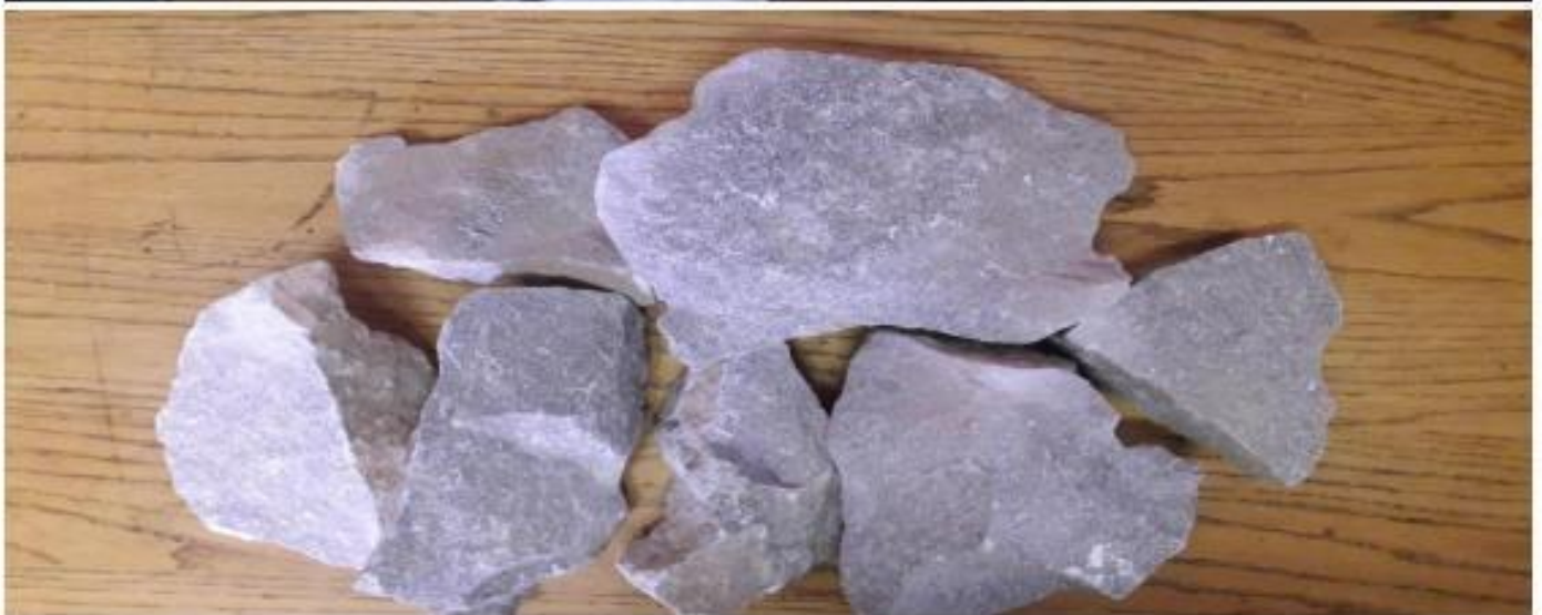
Figures of 2 lithium ore samples showing presents of spodumene obtained from a deeper shaft currently worked on by Artisanal miners at Bepe West 5
