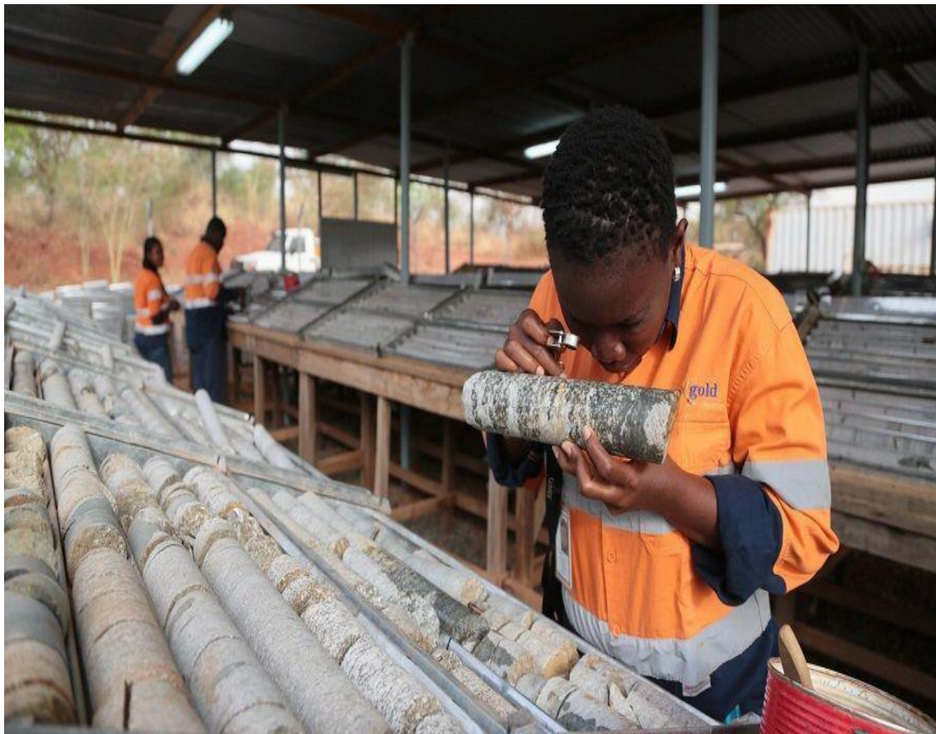
Figure of Drilled Core logging and storage
